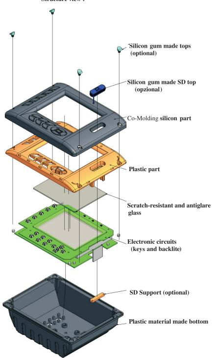
Here is a short description of the Co-Molding technology. This process is employed to make plastic boxes and dashboards for electronic equipment. It involves the employment of policarbonate (PC) in the structure and silicone (Si) materials in keys and covering, meant to be combined in a single body. Remarkable advantages are to be credited to the industrialization of production process, in particular; high rate of protection IP (67/68), design solutions, backlit keys,
